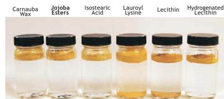
Fig.1 - Flotation test in water.
