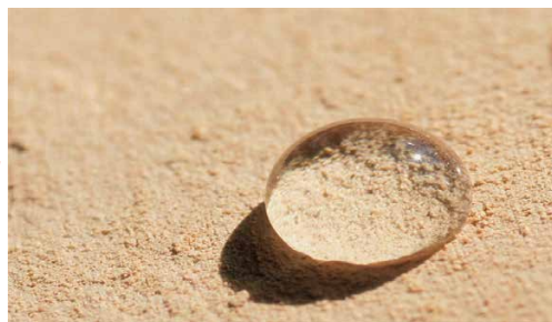
(Oil Droplet on FS Treated Pressed Powder) FS treatment is extremely lipophobic and hydrophobic, allowing it to repel water and sebum on the skin.
