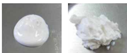
Figure 2. Effect of dispersing pigments using SALACOS® HS-6C (left) versus control (right), in a W/O sunscreen milk
