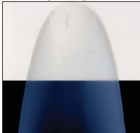
Drawdown of Dispersion (TiO 2 TEL-100 in an Ester)
