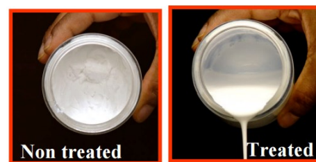
Figure 2: Titanium dioxide (15 nm) flow properties are much improved with surface treatment, PEG-8 Triethoxysilane, yielding lower oil/water absorption and lower viscosity.
